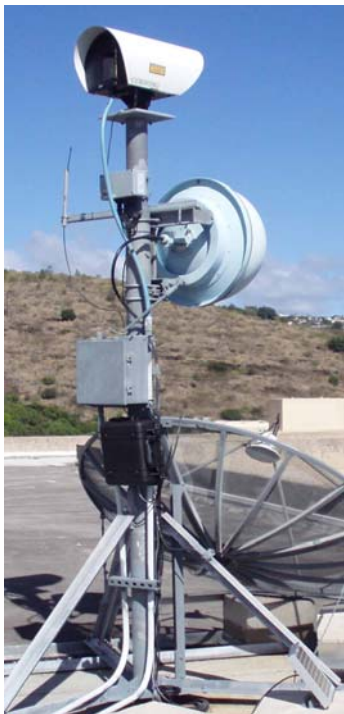
The InteleCell™ unit is inside the black weatherproof case and its antenna is on the left arm of the structure, the solar panel that powers the system is at the bottom right of the
